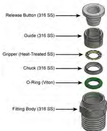
Stainless Steel (SS) Gripper-Style (W) Fitting Materials of Construction
